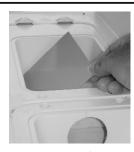
Place plastic plate 110mm x 150mm x 2mm into the rear compartment so that a flat area results here
