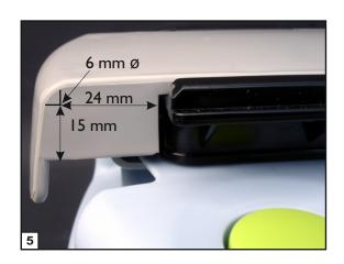
If there is not a hole in the slide handle on the ventilating knob side of the cartridge, this must be provided subsequently.
