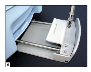
Unlock slide handle and pull on, locate cartridge in reverse position and unscrew the four Torx screws with Torx insert TX 10. Remove slide handle.
