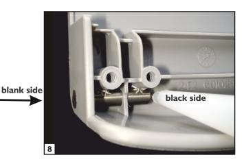
First push control magnet with the face marked black into the hole(direction of the arrow) until this closes with the outer side of the slide handle(black side).
