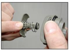
**3** Pull valve actuator out of the valve and remove spiral spring. Insert valve actuator again and push downwards as far as the limit stop.
