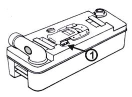
A continually open overpressure valve is located on the fecal tank. This valve is rendered superfluous by the SOG toilet ventilation and must be closed, as otherwise odors occur here during travel, which consequently make their way into the service compartment and hence into the vehicle.
