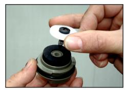
**4** Insert rubber disk - screw valve actuator together with plastic screw (see photo). Insert valve in the cassette again.
