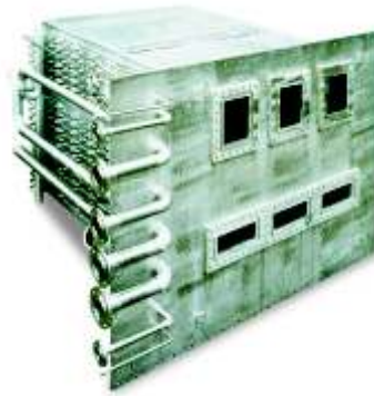
Heat exchangers for air/steam condensation, for aggressive media designed as direct evaporators, made from V 4 A steel, with several cooling circuits for R 23 / R404A cascades and an integral water glycol circuit for de-icing the heat exchanger. Suitable for petrol vapour recovery, dichlorotoluene condensation etc.
